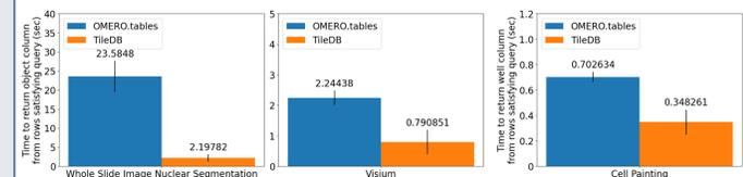
**Figure 7:** Column-major order in TileDB significantly improves the speed of data retrieval from remote tabular datasets when compared with OMERO.tables/PyTables. Visium data in OMERO.tables was smaller due to current column count limitations, so relative improvements are likely even greater.
